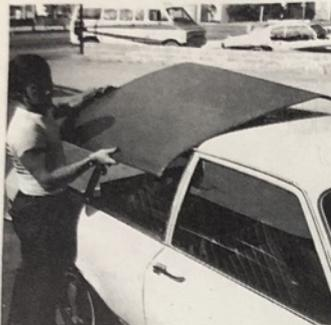
Fit top panel over drain molding edge. To tighten use rubber hammer forcing down on edge of molding.
