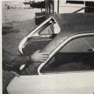
Install rear end sections, file for fit. Slip over drain molding edge and the inner rear door edge.
